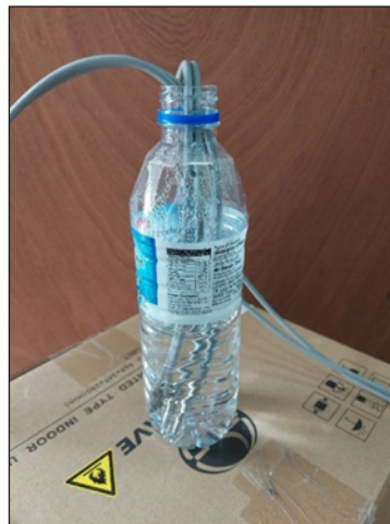
Figure 7. Temperature sensor calibration check in water medium
