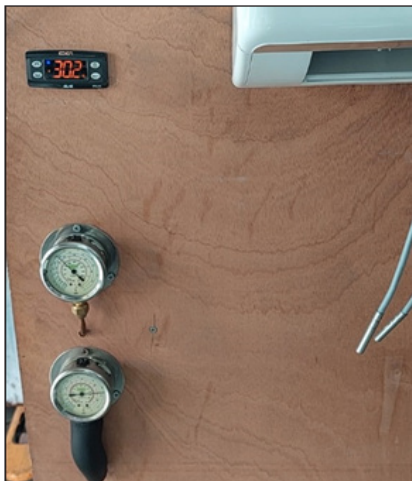
Figure 6. Temperature sensor calibration check in ambient air
